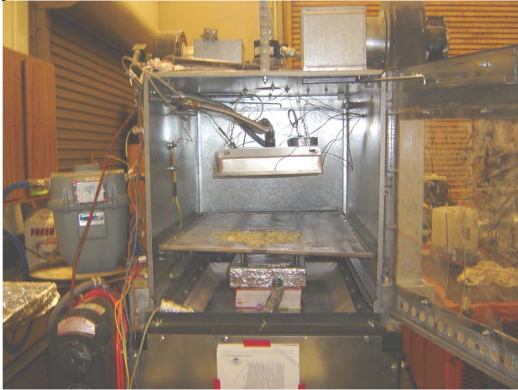
Fig. B1. Catalytic infrared (CIR) set up for drying onions
